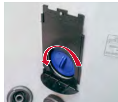
Turn Filters Counter-clockwise to Remove
