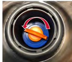
Turn Filters Counter-clockwise to Remove
