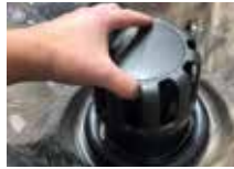
Pull Up to Remove Floater Assembly
