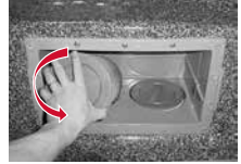
Turn Filter Counter-clockwise to Remove
