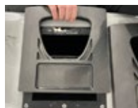
Let the Weir Door to fall back towards the filters when removing the filter housing.
